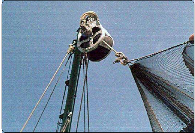
"MACACO" (Power Block).
